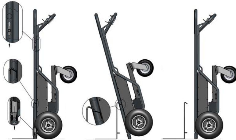
Capture/Release by Leaning Truck Forward and Pulling Release Handle.
